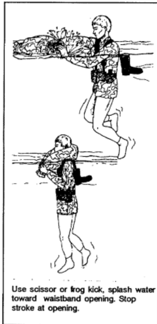
Figure 13 Trousers Inflation - Splash Method
